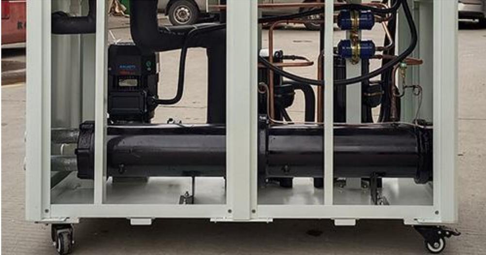
*Shell and tube Condenser for water-cooled fermentation chiller*
